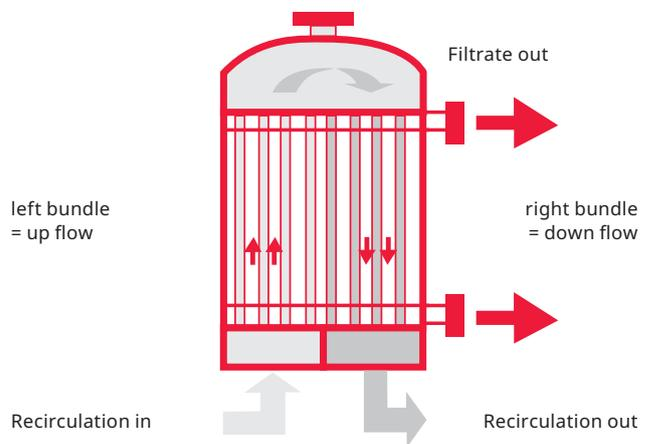
Thanks to this concept, a maximum of packing density and a minimum of pipe connections are achieved. Complete venting and draining is guaranteed by discharging the liquid through the top and bottom plate.
