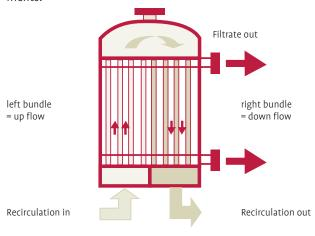
Thanks to this concept, a maximum of packing density and a minimum of pipe connections are achieved. Complete venting and draining is guaranteed by discharging the liquid through the top and bottom plate.
